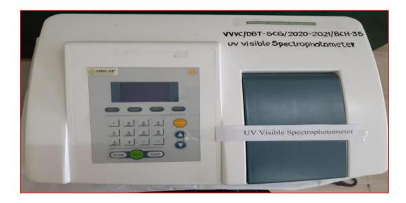
UV-Visible spectrophotometer is used to study the optical absorbance of the thin/thick films or any chemical substance or light absorbance of the systems.
