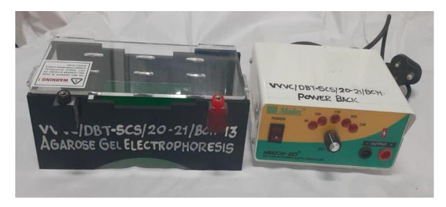
Agarose gel electrophoresis is widely used for separation of DNA and RNA samples in events like restriction fragment analysis, polymerase chain reaction product analysis, checking the integrity of genomic DNA, and purification of nucleic acids.
