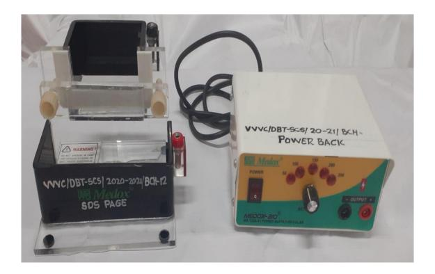
SDS PAGE or Sodium Dodecyl Sulphate-Polyacrylamide Gel Electrophoresis is used for the separation of proteins based on their molecular weight. It is a technique widely used in forensics, genetics, biotechnology and molecular biology to separate the protein molecules based on their electrophoretic mobility.
